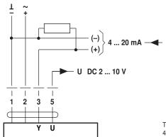
The 500  $\Omega$  resistor converts the 4  $\dots$  20 mA current signal into a voltage signal DC 2  $\dots$  10 V
